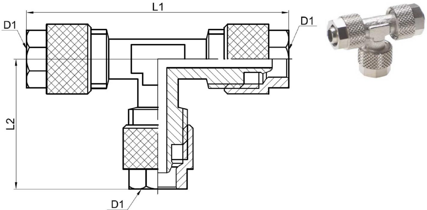
**MATÉRIEL:** LAITON NICKEL PLATED**ØD1:** ØEXT/ØINT TUBE
